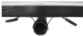
Black/Grey Tank Drain and Valves
